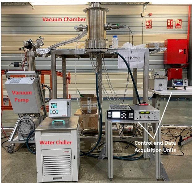
Figure 1: Main components of the ALBA experimental setup for the study of thermal contacts.
