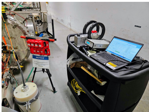
Figure 2: Helmholtz coil and fluxmeter measurement rig in the tunnel next to a set of samples on a tripod. Note the adjacent NDX detector.
