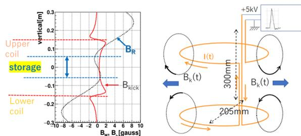
Figure 7: kicker system (right side) and radial field distribution along the solenoidal axis at radial point of 11 cm in red solid line.
