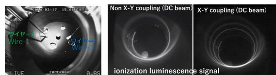
Figure 6: Internal views of storage chamber as well as visualized electron beams.
