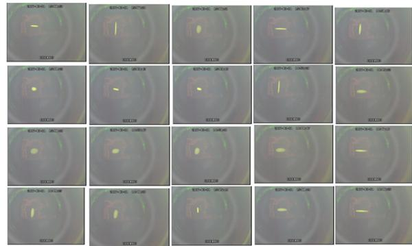
Figure 4: Twenty views of beam cross-section at the end of the straight line, by changing settings of three rotating quadrupole magnets as in Fig. 3.
