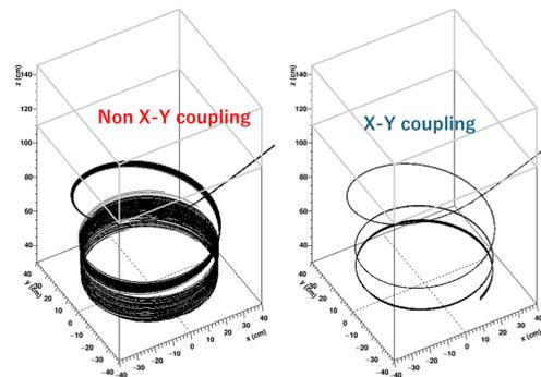
Figure 2: Left: Three-dimensional beam tracking without appropriate X-Y coupling. Right: The same but applied appropriate X-Y coupling with regards to given magnetic field [2].
