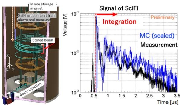
Figure 8: Left: Experimental setup for pulsed beam operation. Right: Signal of stored beam by use of SciFi.
