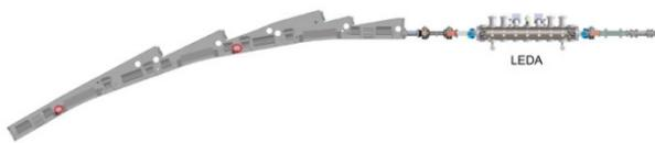
Figure 6: LEDA scraper positions circled in red.
