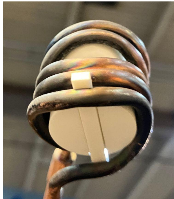
Support post provides alignment
