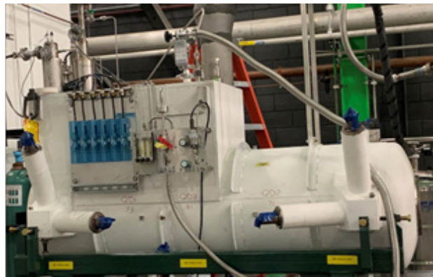
Figure 14: A recently built spare S800-style SC quadrupole triplet for the FRIB experimental beamlines.
