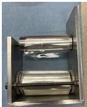
Figure 1: The belt-conveyor-type target.
