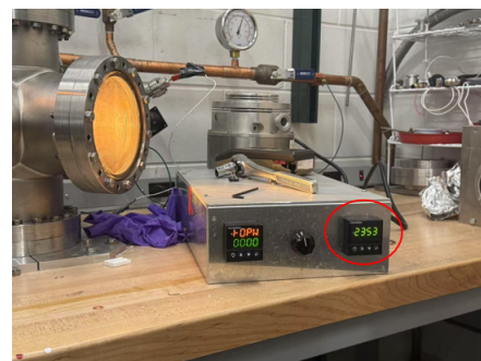
Figure 4: The maximum temperature ever reached in HTO at 2353 °C.
