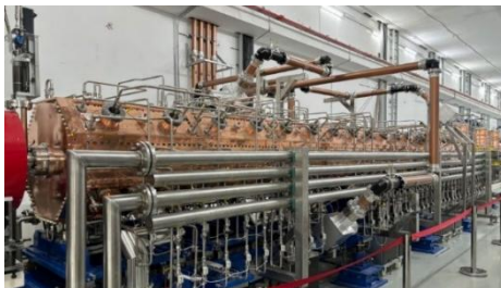
Figure 4: HIAF RFQ have been installed and commissioned.
