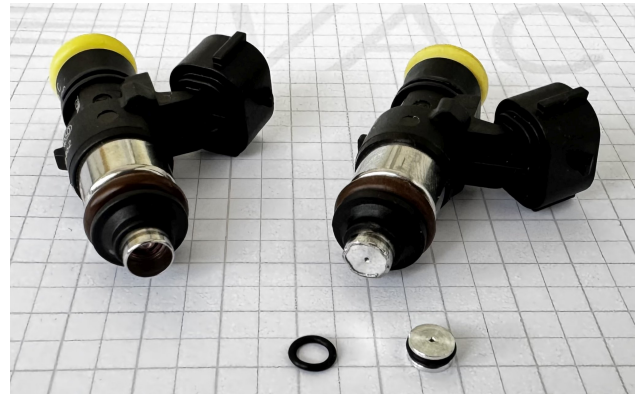
Figure 3: Injection valves used for the pulsed gas stripper. The valve on the right is modified by an orifice with a diameter of 0.6 mm placed in the outlet tube. On the left, an unmodified valve is shown for comparison. In front of the valves are an O-ring and another orifice with O-ring mounted.
