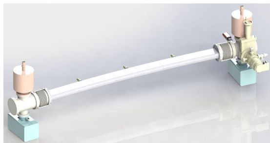
Figure 5: Ultimate vacuum and life testing device for titanium alloy lined vacuum chamber.
