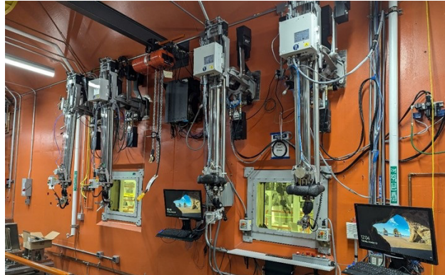
Figure 13: Two sets of remote handling manipulators for the FRIB target hall.
