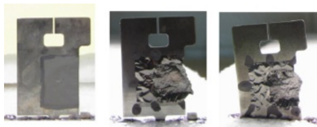
Figure 3: Damage produced by a ^{208}\text{Pb}^{27+} beam, 8.1 MeV/u, on Diamond-Like-Carbon (DLC) stripper foils in the NSCL K1200 Cyclotron [4].
