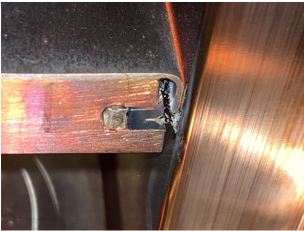
Figure 3: Damage at the transition between tuning plates and stems after operation with 150 kW/m.
