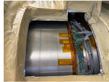
Figure 10: Inside the helium enclosure, a view of a singlet wiring.
