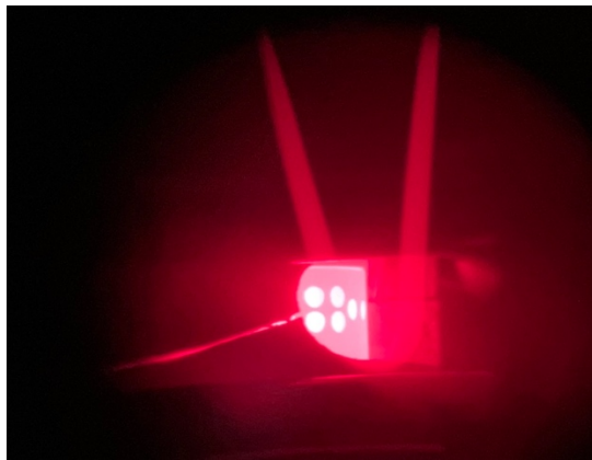
Figure 4: Thermal imaging of the channel holes of an elongated susceptor design looking through the aperture of the surrounding insulator, where lighter colors indicate higher temperatures. The circular holes can be seen to be hotter than the surrounding susceptor, making them less likely to clog from material condensation.
