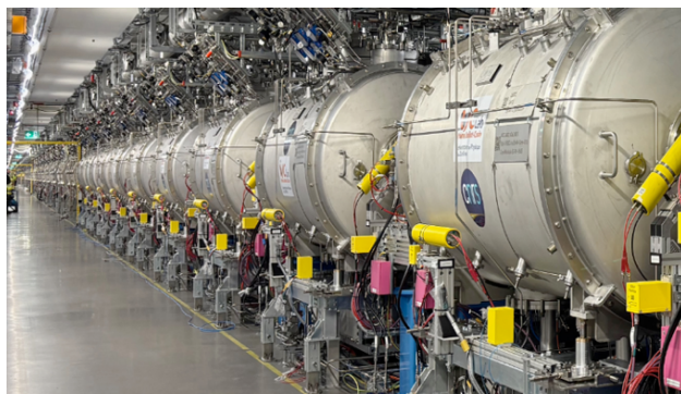
Figure 1: Installed Cryomodules in the linac.
