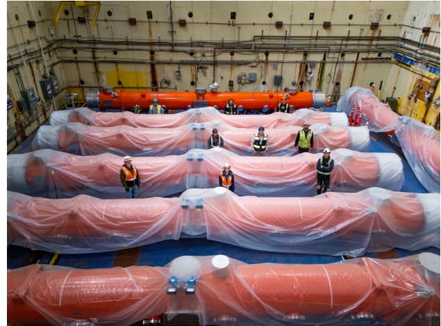
Figure 12: LCLS-II-HE cryomodule storage pictured with installation team. Photo courtesy of SLAC National Accelerator Laboratory.
