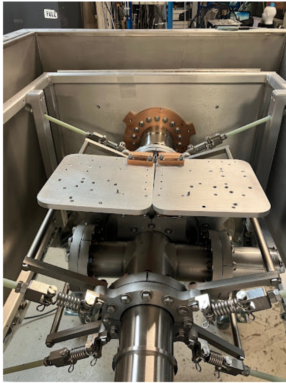
Figure 3: Post-clean room assembly of 5N Al split rings and 5N Al plates to be coupled to cold head second stages.
