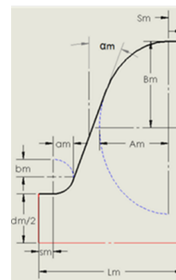
Figure 3: The main parameters of an elliptical cavity.
