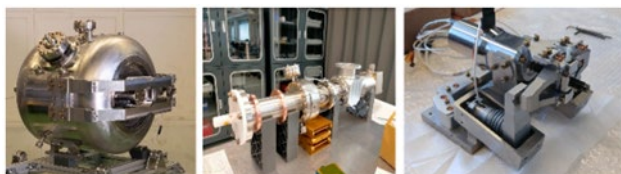
Figure 1: Pictures of the three types of components: a SSR2 resonator (left), a power coupler (center) and a tuner (right).
