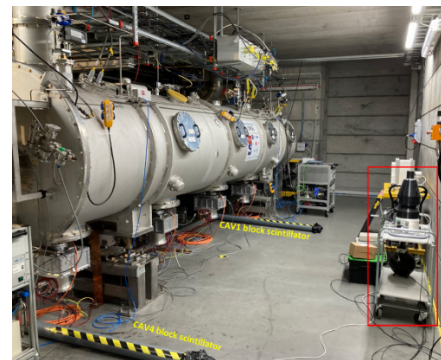
Figure 1: Two plastic scintillator blocks are placed on the ground close to cavities 1 and 4. The detectors in the red insert are described in the figure below.
