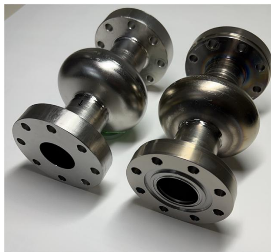
Figure 1: Developed 3 GHz single-cell cavities; left: cavity with low-RRR flange, right: cavity with NbTi flange.
