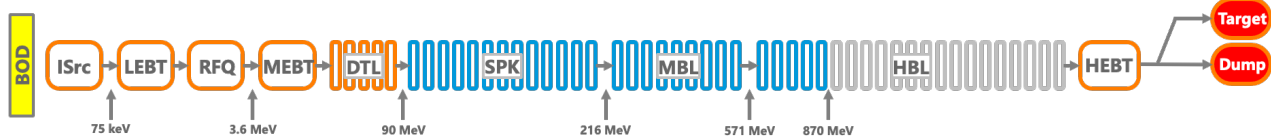
Figure 2: The ESS Linac configuration for the Beam on Dump phase.
