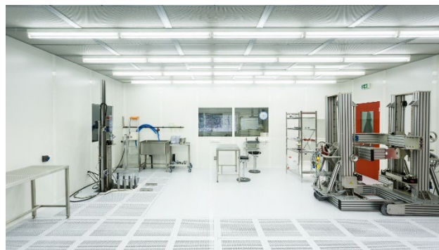
Figure 1: Picture of the ISO-4 dedicated cleanroom for cavity cleaning and assembling of the SUPRATEch facility that shows the HPR mechanical system on the left, and the cavity manipulation system on the right.
