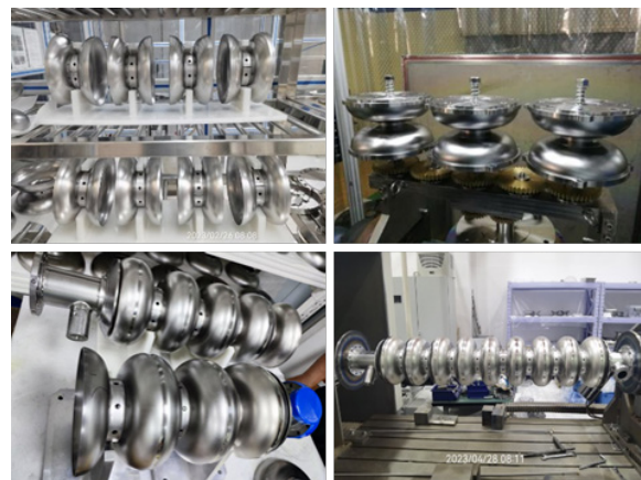
Figure 2: Machining and EBW of cavities.
